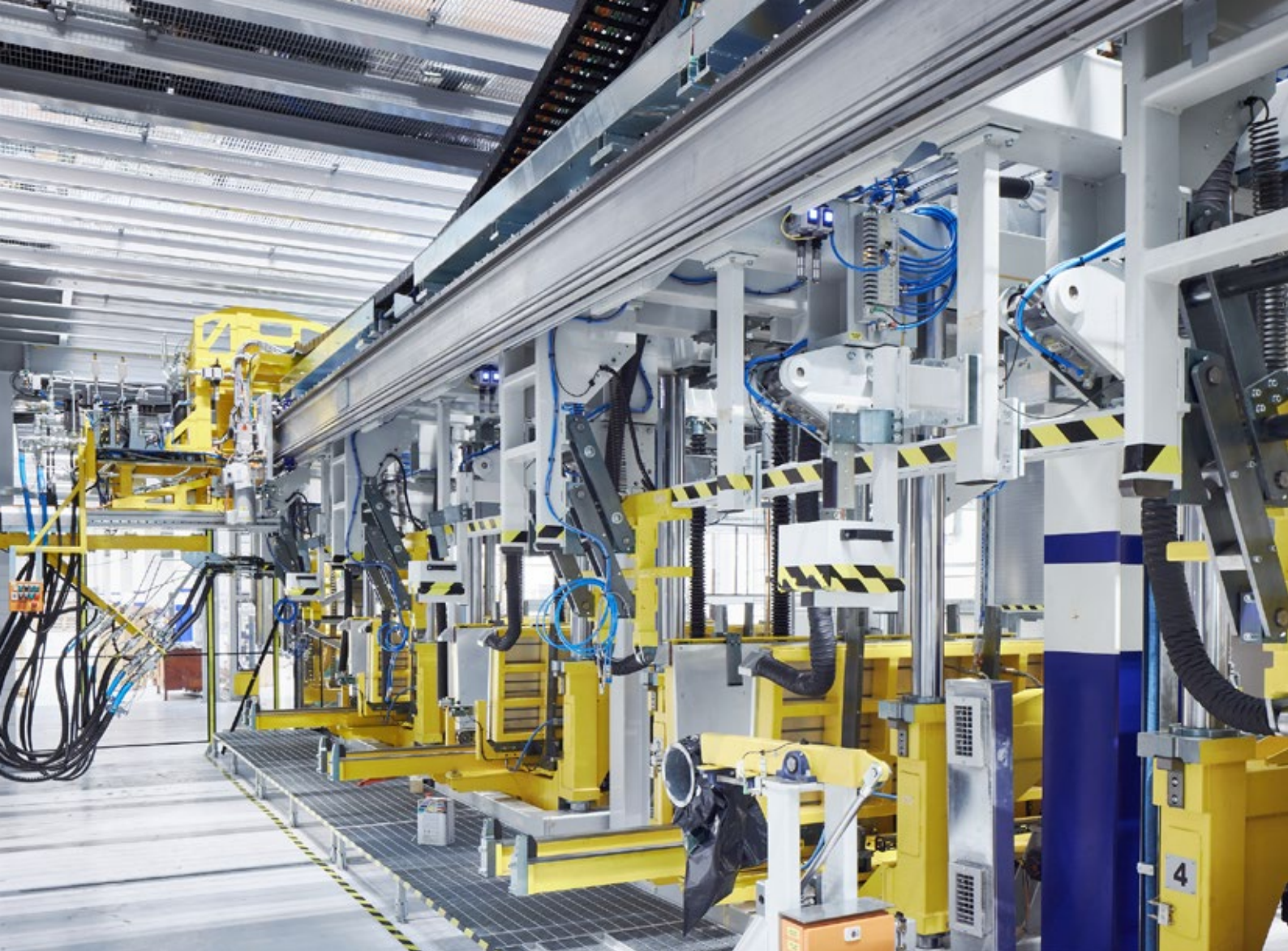
Container foam facility for insulation and reinforcement of refrigerators
