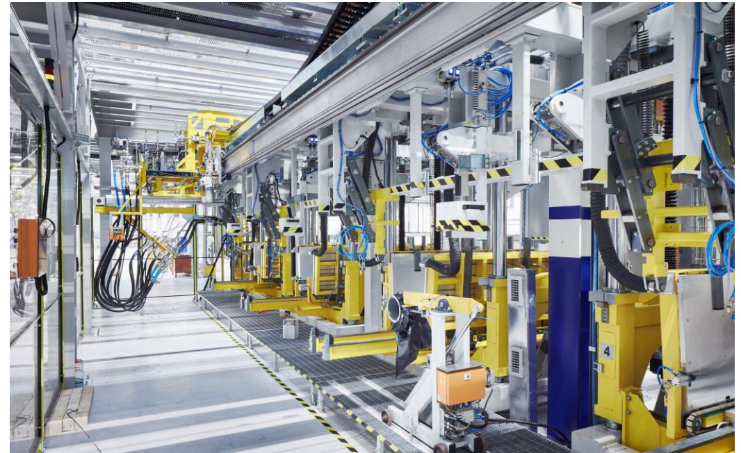
Container foam system for isolation and reinforcement of refrigerators
